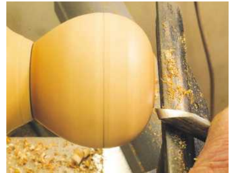
▲ Pic.8 If you present the tool to the wood like this the tool will catch, causing a big spiral cut up the timber; the tip of the tool should not come into contact at all
